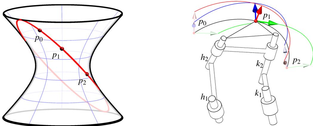
Figure 2: Three-pose synthesis of a four-bar linkage.
