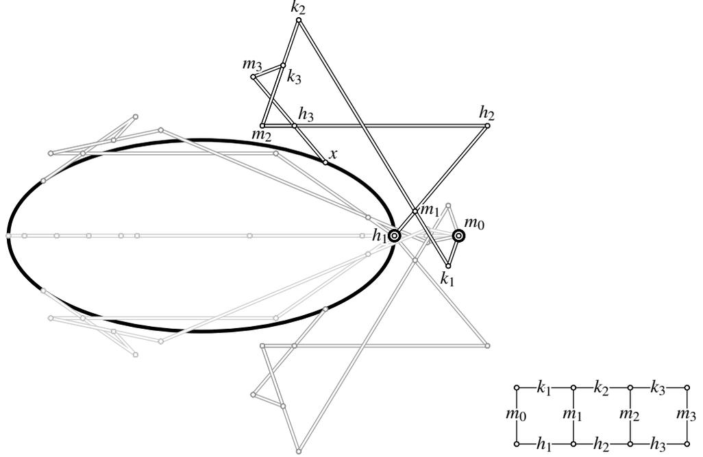
Figure 6: Linkage to draw an ellipse and link graph.
