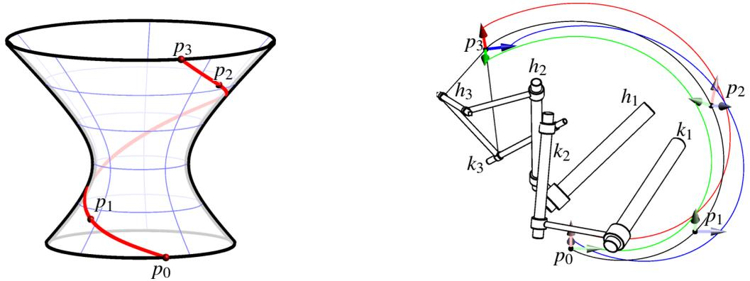
Figure 3: Four-pose synthesis of a six-bar linkage.
