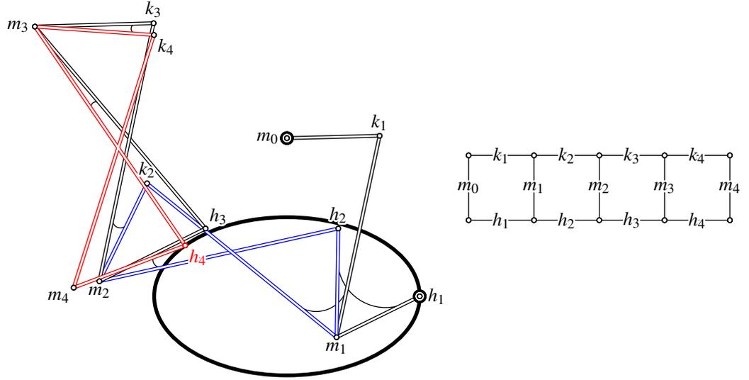
Figure 5: Linkage to generate an elliptic translation and corresponding link graph.
