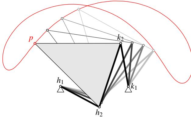
Figure 1: Anti-parallelogram linkage.
