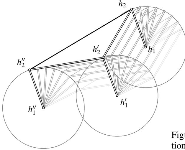
Figure 4: Three different factorizations of a circular translation.
